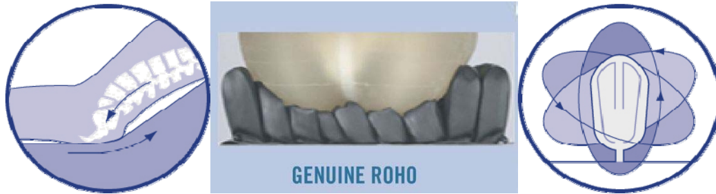
The design of the ROHO cell conforms to the shape. Shear in a bed with bed head raised (left), image of cells compensating to reduce shear (middle), and how the cells move (right)
